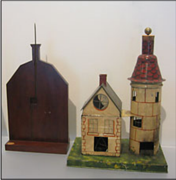
These 18th century 'thunder houses' were used in Harvard classes to demonstrate the effectiveness of Franklin's most famous invention, the lightning rod.
