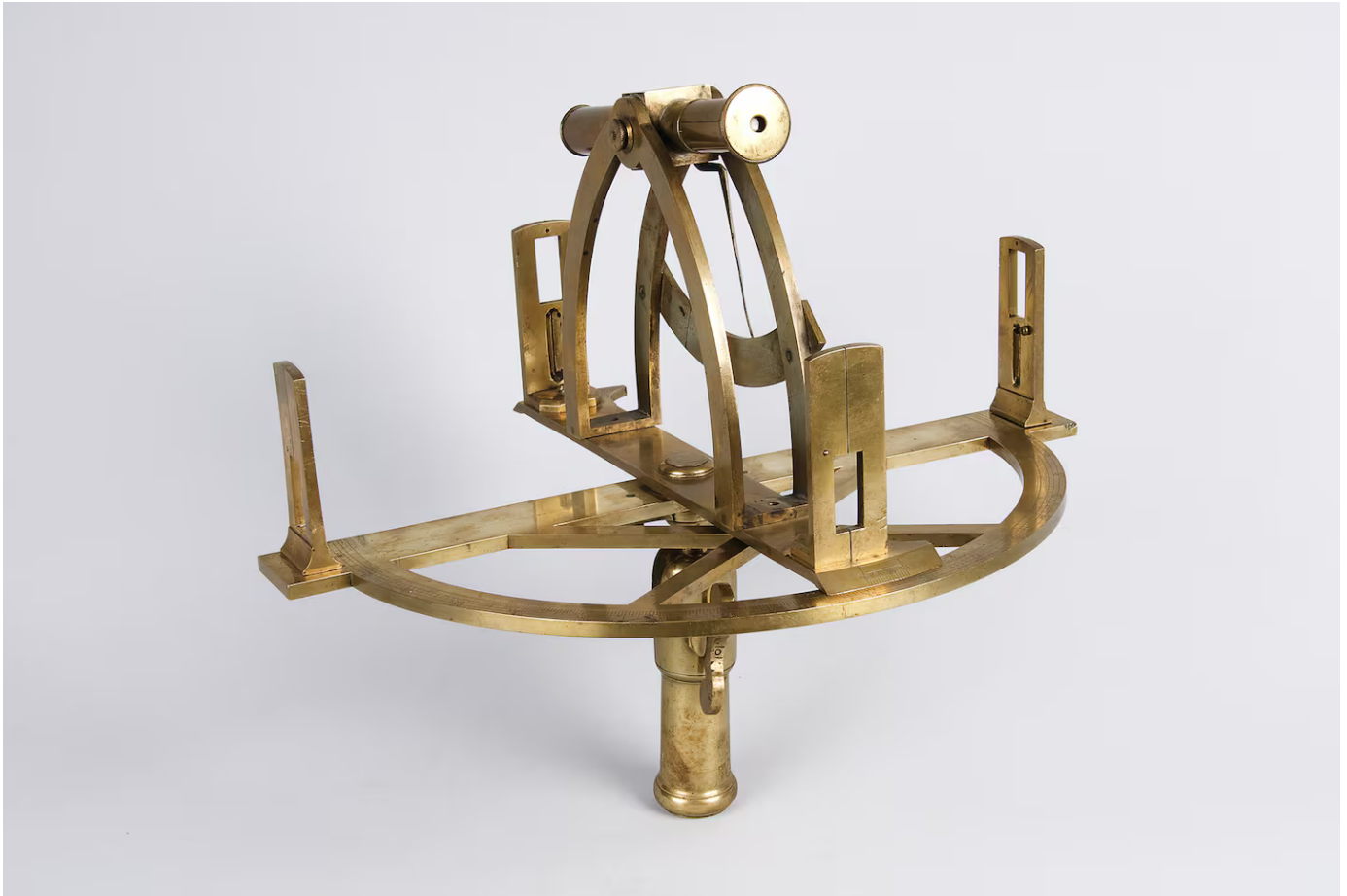
Altazimuth graphometer by Muerand, Paris, 1780. HARVARD COLLECTION OF HISTORICAL SCIENTIFIC INSTRUMENTS
