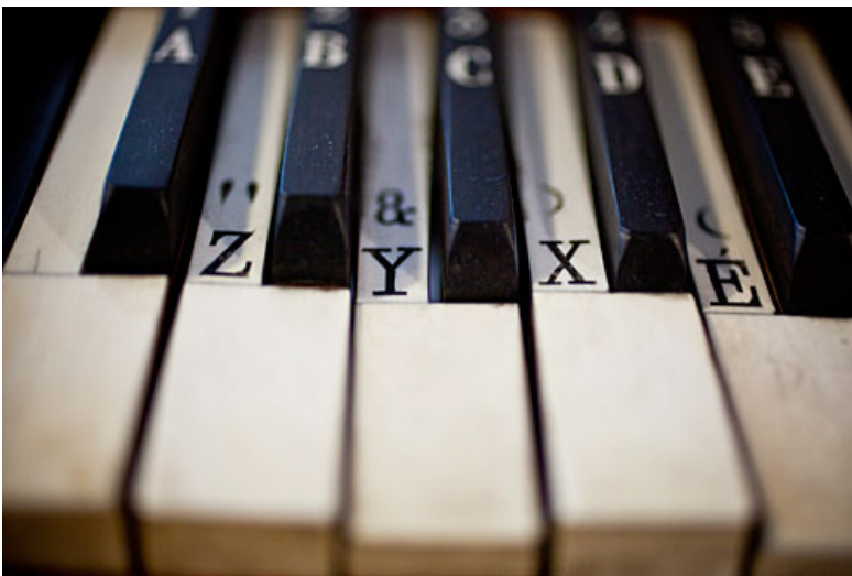
A close-up of a Hughes-type printing telegraph by Louis-Clément Breguet, c. 1875.
